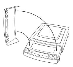
**5** If you use in-use protective cover, peel off the paper to expose the adhesive on it, then fit it on the display and key part. Press the adhesive parts gently.
