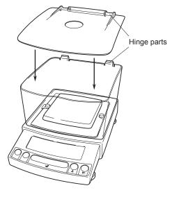
(4) Place windbreak lid on top of windbreak main fitting the hinge parts.
