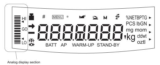
The UW/UX series balance has an analog bar graph located on the left side of the display. This graph can be conveniently used for checkweighing or cumulative weighing.
