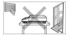
Air flow from air-conditioner, open window, or ventilator
