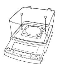
(2) Fit windbreak main on top of the balance main body, and fasten it with two fixing knobs.
