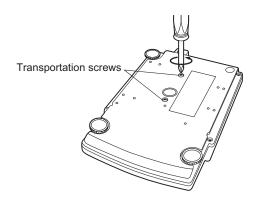
Referring to the explanation label on the bottom of the balance, turn the two transportation screws counterclockwise until they tighten again. (UW only)
