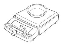
1 If a weighing vessel (tare) is used, place it on the pan and wait for the stability mark to illuminate.
