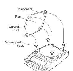
4 Install the pan. With small pan model with minimum display of 0.001g, the standard windbreak is also installed here.
