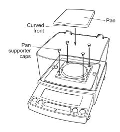
(3) Insert the four pan supporter caps into the holes in the top of the balance. Place the pan on them. Positioners on the pan must fit pan supporter caps.
