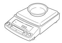
**2** Press the **[O/T]** key to zero the display. (This operation is called "taring".)
